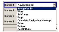
**Navigation Bit** A marker signal is generated for every navigation
