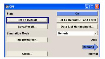
The upper section of the menu is where the GPS digital standard is enabled and the default settings are called.
